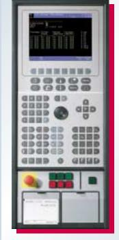
Ergonomics in detail: The Ergocontrol terminal can pivot for convenient access to the injection unit.
