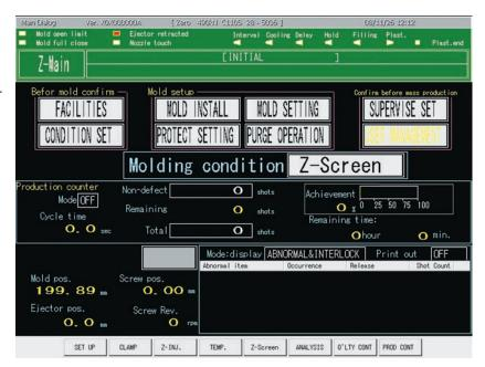
The Z-Main Screen allows the operator to easily move to set screens. In addition to One Process = One Screen, the flow of condition setting can be easily followed without referring to the manual.
