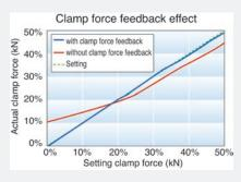
The MCM System working together with the Clamp Force Correcting System achieves exceptional stability even at low clamp force settings.
