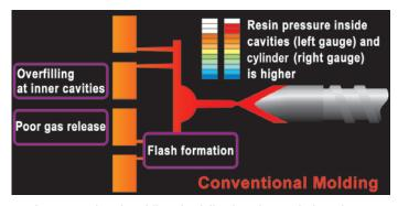
In conventional molding, by fully charging resin into the mold cavities, overfilling and compression occur at the inner cavities and gases are trapped.
