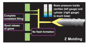
In Z-molding, the FFC System restricts screw position to optimize the flow front. Problems associated with overfilling and trapped gases do not occur.
