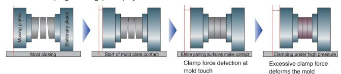
Precision clamp force detection (using a tie-bar-mounted strain gauge sensor) and the feedback control capabilities of the Minimum Clamping Molding (MCM) System determine the minimum force required at mold touch. Using this system can avoid excessive clamp force which can result in mold deformation and poor release of gases.
