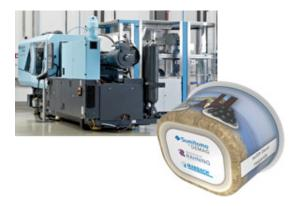
The Marbach-developed process uses a "full cover label placer" that inserts the banner and base label in a single stroke. Previous IML solutions required a partition on the container base that meant that full coverage with the label in the injection mold was not possible.
