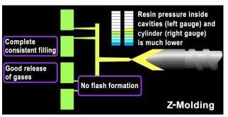
In Z-Molding, the Flow Front Control system optimizes the flow front. By achieving complete, low-pressure filling, the problems associated with overfilling and trapped gases do not occur.
