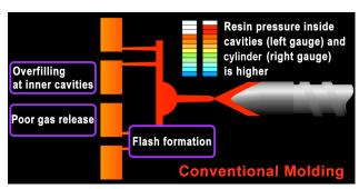
In conventional molding, by fully charging resin into mold cavities, overfilling and compression occur at inner cavities and gases are trapped. At lower pressures, short shots occur.
