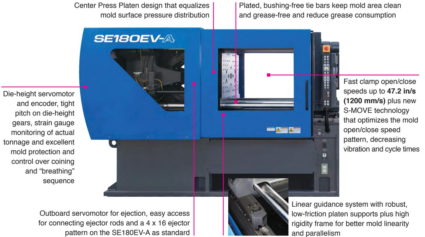
For clamping, the SEEV-A combines advanced servomotor technology for clamping and ejection, fast clamp speeds and the new S-MOVE technology (see below), a rugged and field-proven, double-toggle clamp design and our unique Minimum Clamping Molding (MCM) System (next page) which helps avoid flash, burn spots and shorts shots, and can reduce mold wear, cycle time and power consumption.
