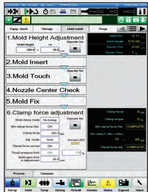
SPS provides a simple, one-page, step-by-step guide for mold installation.
