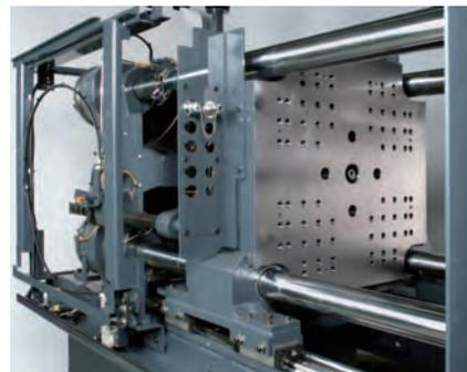
All SEEV-A model sizes were designed with ample tie bar space, in a square configuration, to accommodate larger side-entry molds.
