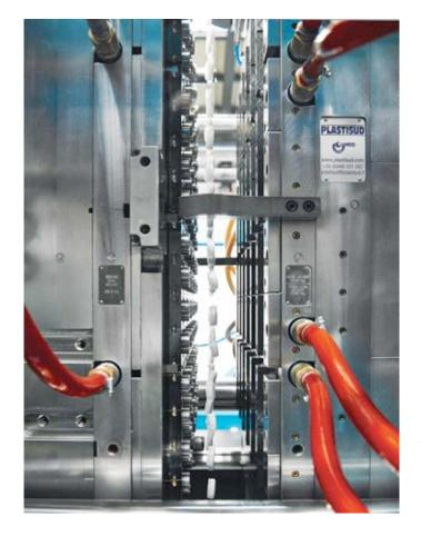
A new generation of high-speed molds combines advanced cooling design with Plastisud hot-runner technology specially engineered for high throughput.
