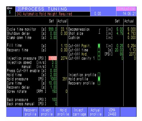
3) Return to screen 83 SETUP and select "Pressure type" Spec. (Specific = plastic pressure).
